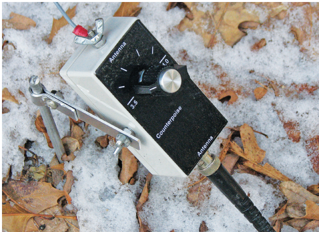
Figure 3 — The matching network mounted directly to the ground rod with the antenna connection at the top of a plastic case and the coax feed connected at the case bottom. The tuning dial is calibrated to enable rapid setup and frequency adjustment.
